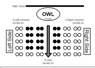
Top-down example of an OWL installation, demonstrating how turning off columns and rows affects the infrared
